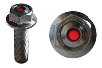
Airfield Lighting Systems Ltd (ALS) have launched SmartBolts - a Visual Indication System that turns the top head of a bolt from red to black as you tighten it. SmartBolts give you peace of mind that your bolts are at the correct tension vital for Airfield safety. They can be easily retrofitted to existing runway lighting systems and do not need to be replaced with every inspection, saving you money and time.
